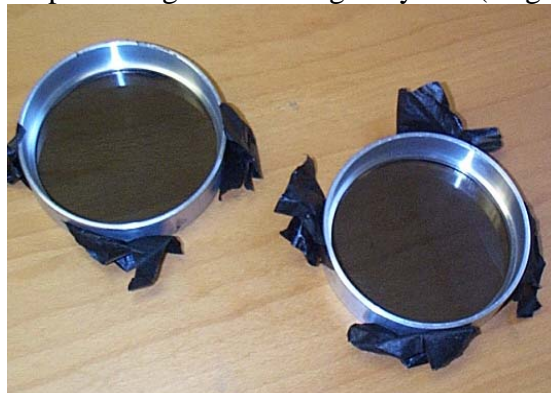
Figure 8. The original polarizing films damaged by heat(1 st generation polarizers).
