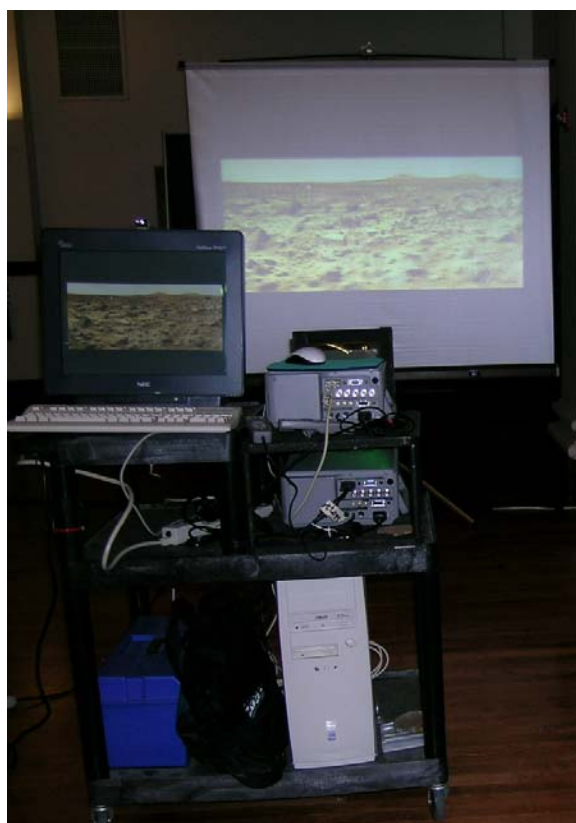
Figure 13. Two different views of the portable cart housing the Cyviz, PC with graphics card, and mounted polarizing films (1 st generation system), and the portable silvered screen.
