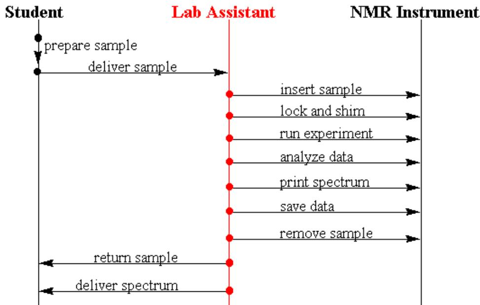
**Figure 1.** Prior to implementing automation, NMR spectra were run by lab assistants.
