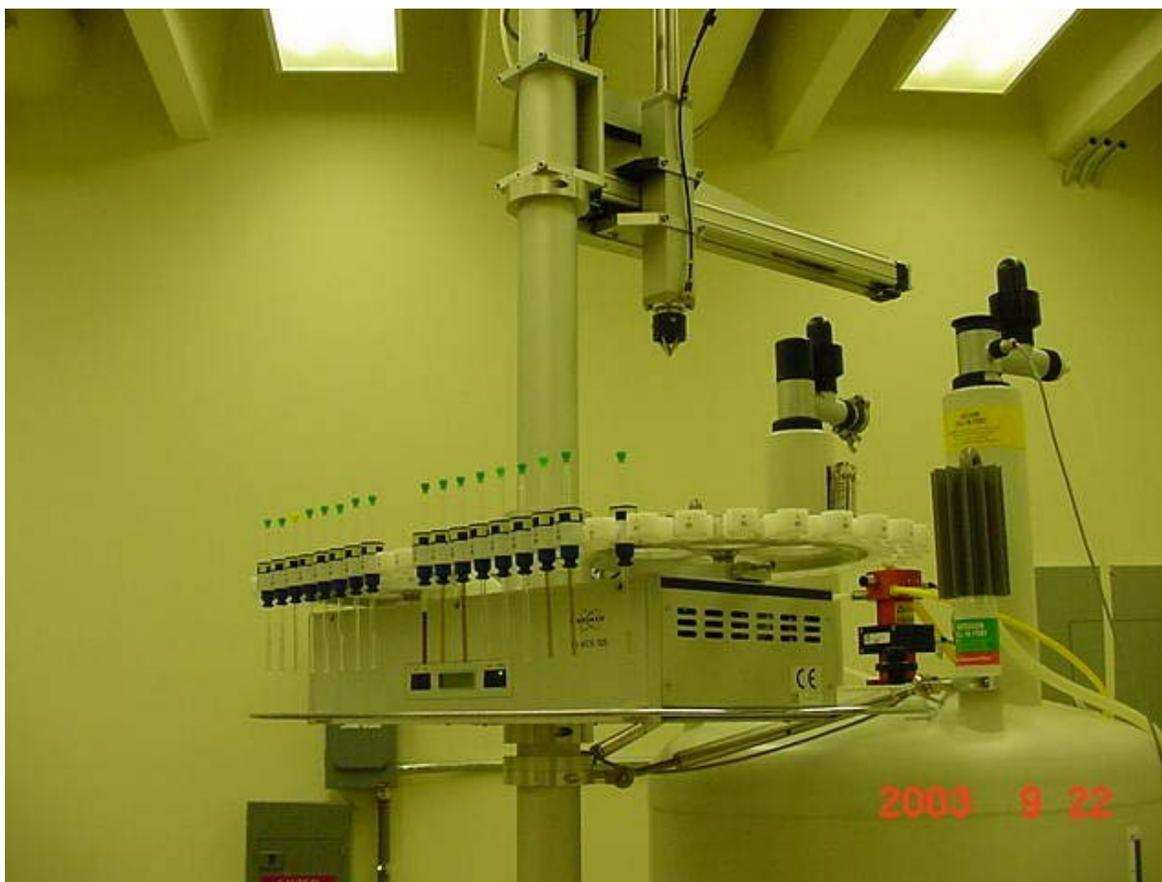
**Figure 8.** Bruker 120-position automatic sample changer (BACS-120) with two concentric rings of sample positions.
