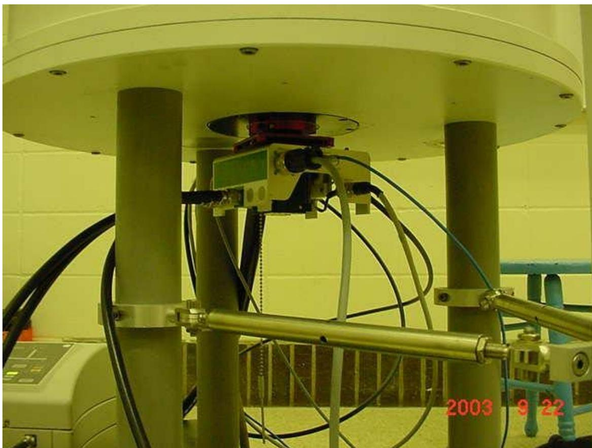
**Figure 7.** Bruker automatic tuning/matching Z-gradient probe.
