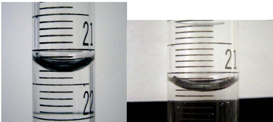
These two were taken with a Canon Elura 2 MC digital video camcorder, the video was converted to a photo. My eye doesn't show the meniscus as sharp as the photo on the left, but using the card gives me better contrast than shown in the photo on the right using a buret reading card.
