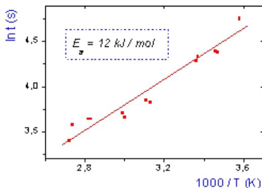
The slope of this graph results in an apparent value of the activation energy for the range 5 - 95°C of  $E_a = 12 \pm 1$  kJ/mol.
