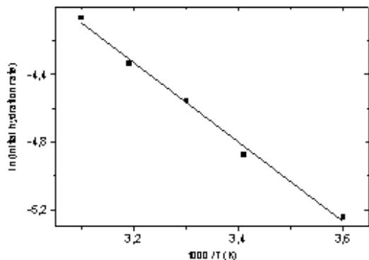
Fig. 5. Graph of natural logarithm of the initial rate of hydration (g water / (g initial wt.·min)) as a function of reciprocal Kelvin temperature.
