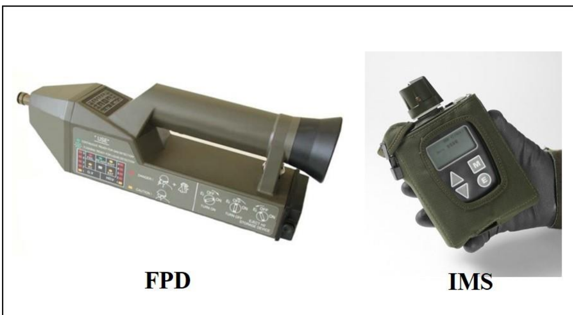
Figure 4: Flame Photometric Detection (FPD) and Ion Mobility Spectrometry (IMS) chemical agent monitors.
