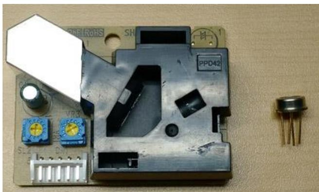
Figure 4 –Shinyei PPD42NS PM<sub>2.5</sub> Sensor (left) SGX MiCS 2710 NO<sub>x</sub> Sensor (right)
